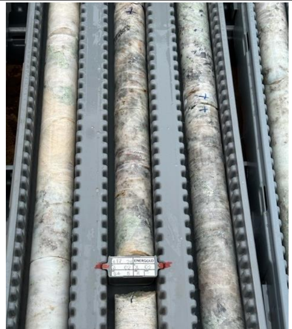
Figure 13: Core from infill drilling at Colina showing medium sized spodumene crystals
