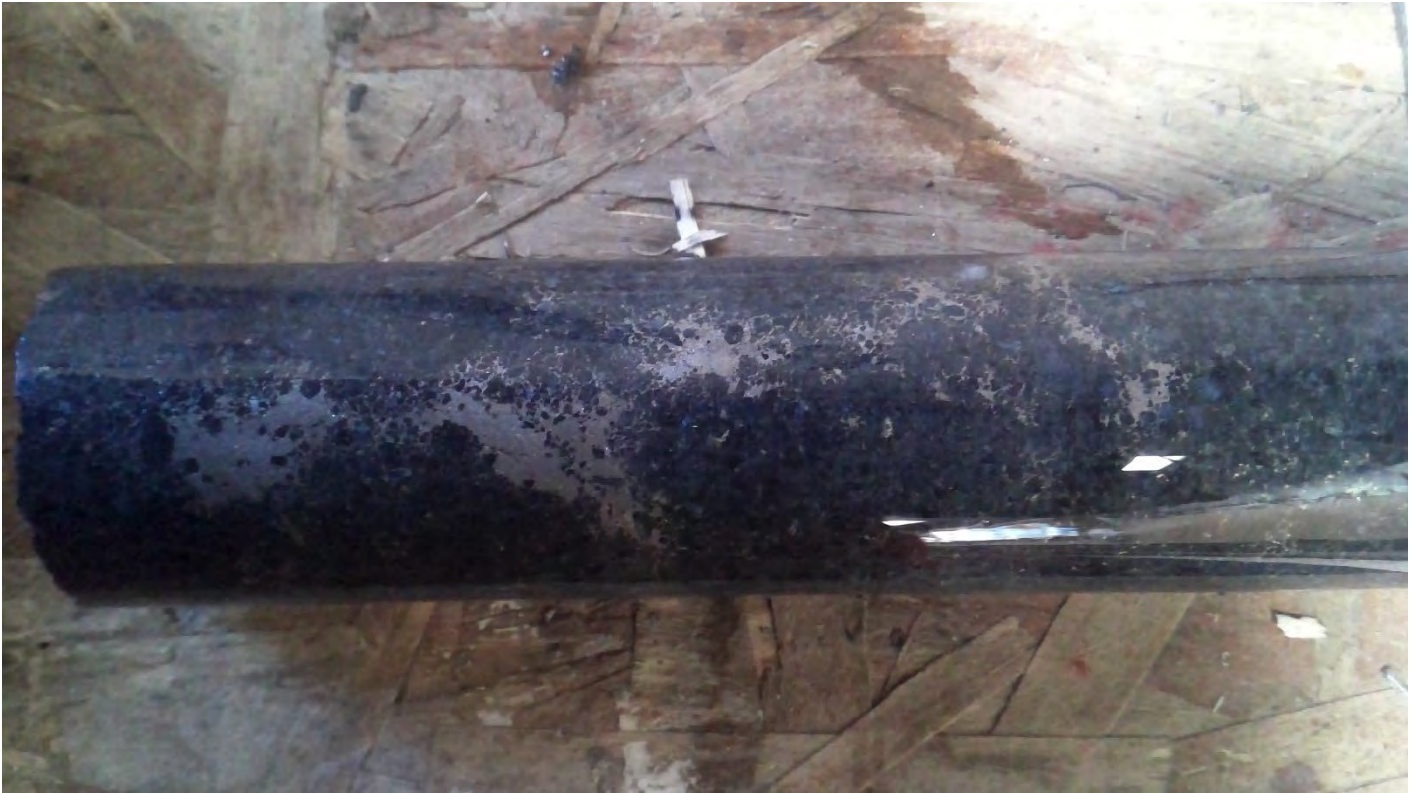
Figure 40. Cumulate textured olivine gabbro with interstitial Po
