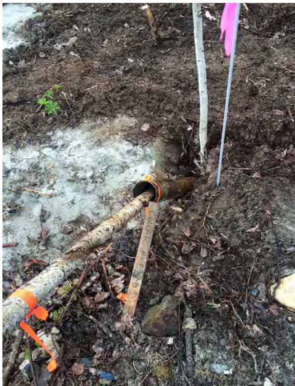
Photo 3. 2015 Crystal Lake Drill Hole Collar
